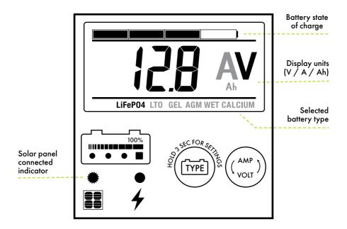
When the unit powers on it will run a self-test sequence as follows:
