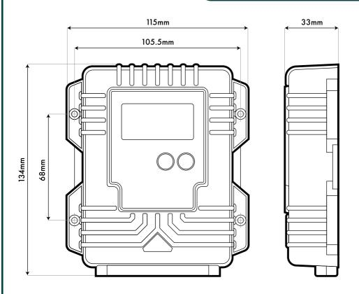
This product can be permanently attached to any flat surface using four self-tapping mounting screws (not included). Simply mark the area you would like to affix the regulator to according to the above diagram and if necessary, predrill holes for the screws to fasten in.
