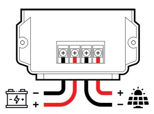
The solar regulator has 4 terminals which are clearly marked 'Solar' and 'Battery'. Refer to the wiring diagram as shown above.
