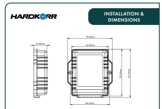
If you wish to permanently mount the solar charge controller, the easiest way to do so is to use two spacers and self-tapping screws (not supplied). Ensure you mount to a flat surface.
