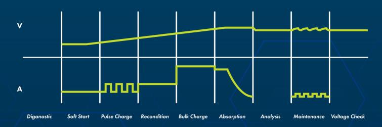
Our chargers come with an automatic 9-stage charging algorithm, designed to charge your batteries quickly and maximise their longevity.
