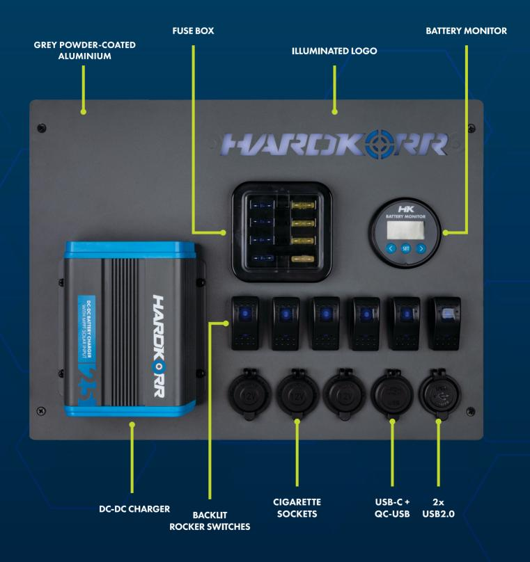
Charge your batteries while you drive or from the sun. The charger comes with an inbuilt 25A/40A MPPT solar regulator which has been pre-wired to a dedicated solar Anderson input on the side of the box. Compatible with LiFePO4, AGM, SLA, Gel, and Calcium batteries, it's the perfect addition to any 12V touring setup.
