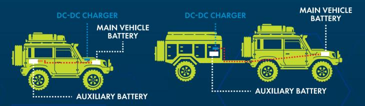
This DC-DC Charger will charge your batteries at up to 25A/40A per hour. Compatible with vehicles running either a standard or smart alternator, it uses a three-stage charging algorithm to optimise power delivery to your auxiliary battery in order to prolong its lifespan.
