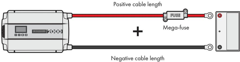
**TOTAL CABLE LENGTH = POSITIVE CABLE LENGTH + NEGATIVE CABLE LENGTH**
