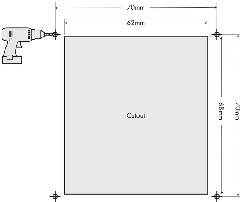
3. Drill 2mm holes in the marked mounting points (or simply leave the points marked) and cut a hole in the surface of the mounting location according to the above diagram.
