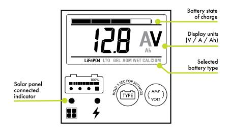
When the unit powers on it will run a self-test sequence as follows:
