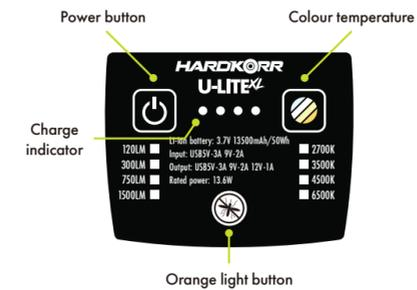
Double press the power button to turn the light on. The light will remember the last light setting that was used. Press the power button shortly after the light is turned on to cycle through the different brightness modes. If the button is not pressed for more than 5 seconds, the next press will turn the light off.
