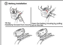
Install the battery correctly then close the cover.
